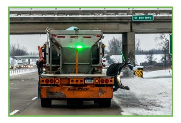
Michigan law allows state and local road agencies to equip their maintenance vehicles with flashing or oscillating green lights in addition to the traditional amber lights. The green lights will only be activated when road work is taking place. Private contractors are not allowed to display green lights on their vehicles.
